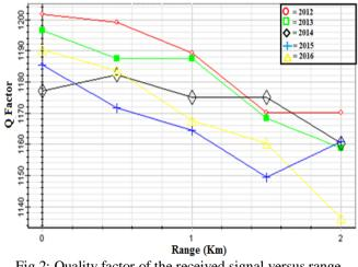
Fig 2: Quality factor of the received signal versus range (different years)
